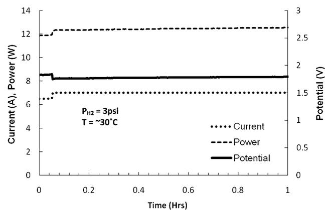
Fig. 9 – Fuel cell stack performance for approximately 1 h of constant operation.
