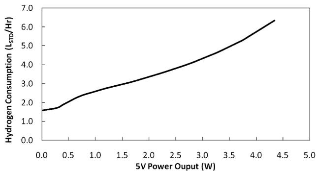
**Fig. 11** – PEM Fuel Cell System hydrogen consumption with respect to power output.
