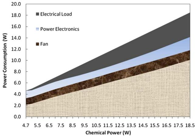
**Fig. 10** – Power summary of portable fuel cell system with only a 5 V load varying from 0 to 4.25 W.
