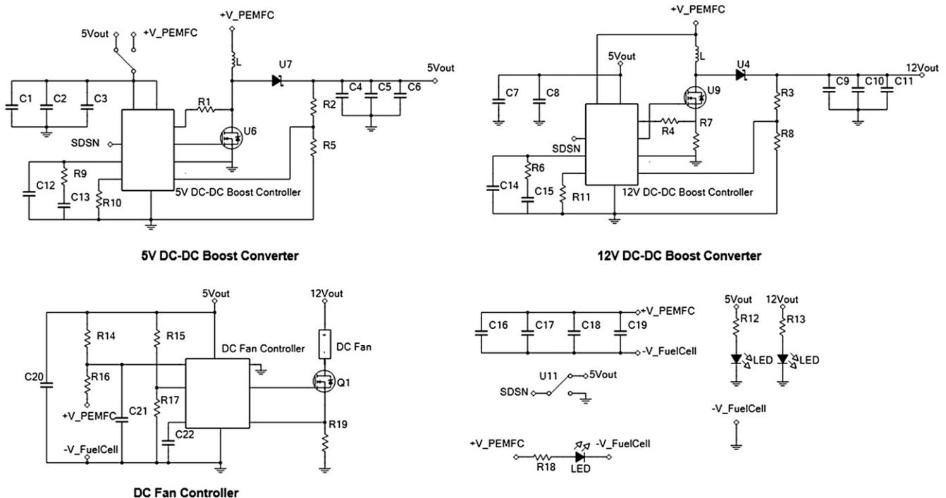
**Fig. 6 – Schematic of Power Electronics and Fan Controller.**
