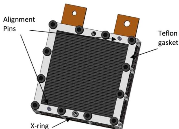
Fig. 4 – CAD model for Teflon gaskets on the cathode side.
