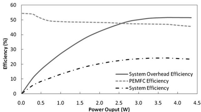
**Fig. 12** – Power and efficiency curves for fuel cell stack and total power system with a varying 5 V load from 0 to 4.25 W.
