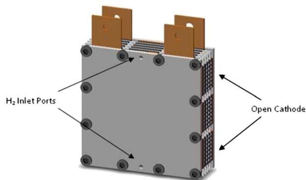
Fig. 1 – CAD model used for design of the fuel cell stack.
