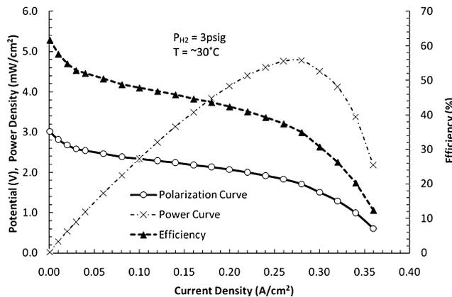
Fig. 8 – Polarization curve of the IAHE-OU fuel cell stack for steady state operating conditions.
