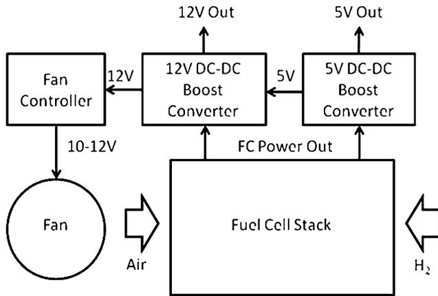
**Fig. 5 – Block diagram of entire fuel cell stack power system (excluding hydrogen storage device).**
