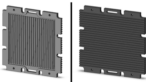
Fig. 3 – Bipolar plate anode flow channel design (left) and cathode flow channel design (right).
