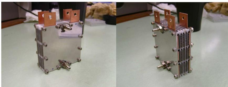
Fig. 2 – Images of PEM Fuel Cell Stack.
