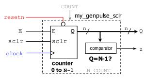
• The output z can then be connected to every flip flop, counter, and register whose rate of operation we would like to modify. This way, we get the same effect at modifying the clock frequency to  $f/_N$ , where *f* is the frequency of the input clock.
