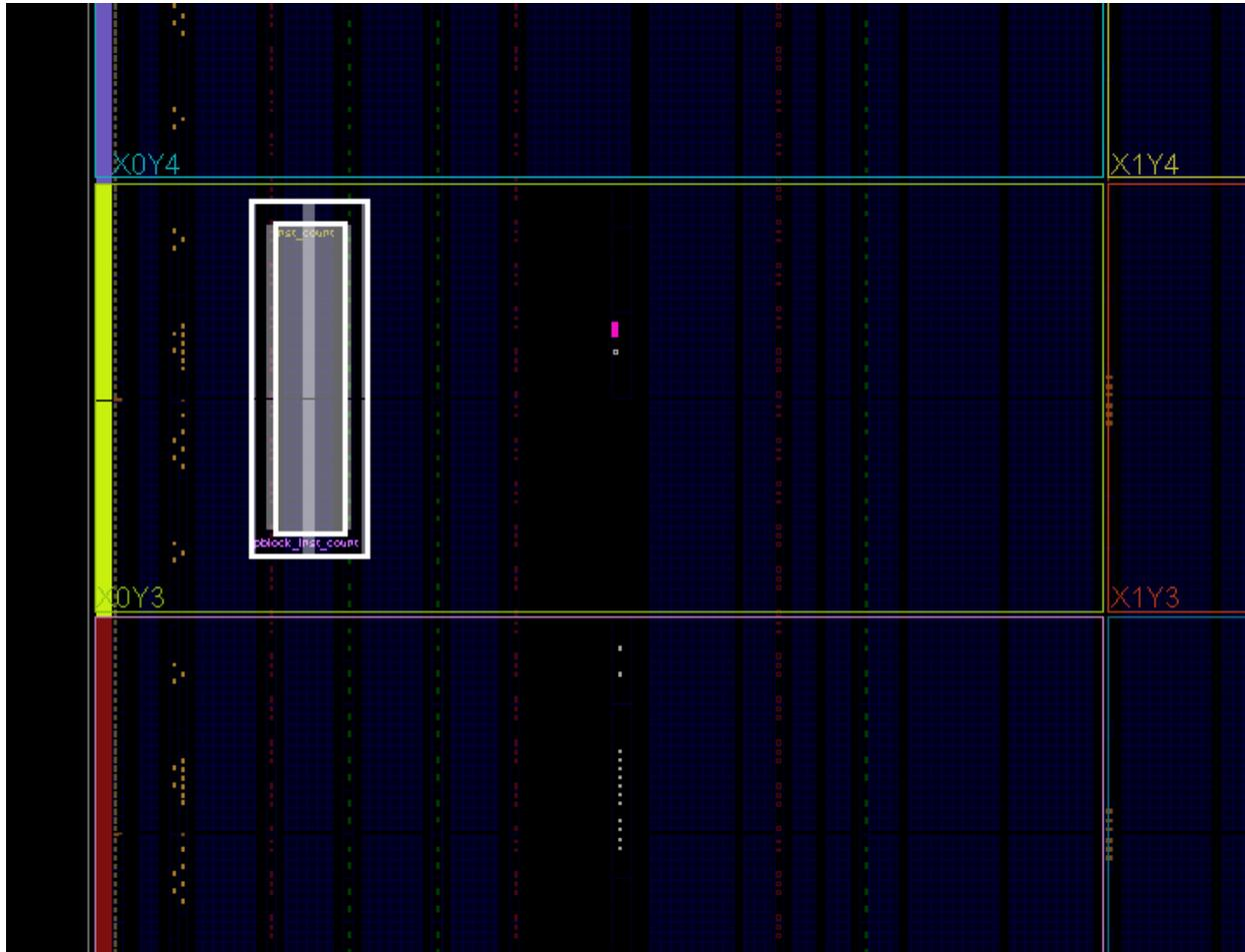
**Figure 1: Pblock for the `inst_count` Reconfigurable Partition**
