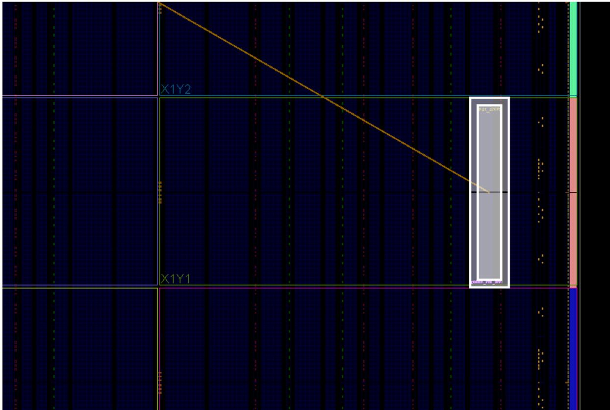
**Figure 4: Pblock for the aligned `inst_shift` Reconfigurable Partition**
