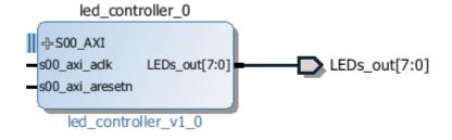
Figure 4.10: led\_controller block with external port
