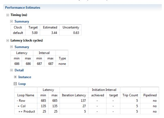
The synthesised design has an interval of 687 clock cycles. Each input array contains 25 elements (as it uses 5x5 matrices) and so this suggests roughly 27 clock cycles per input read. We can now run a C/RTL cosimulation to ensure that the synthesised RTL behaves exactly the same as the C++ code under test.
