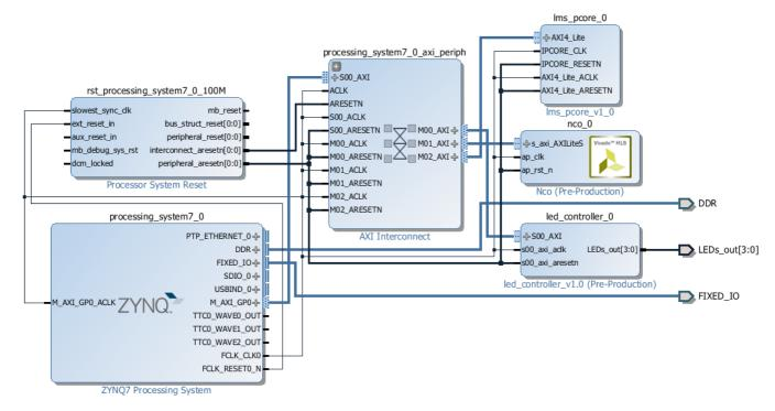
Figure 5.13: Zybo end of exercise block diagram
