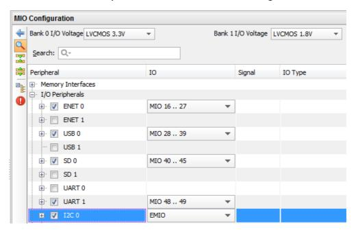
Figure 5.19: Configuring the I2C interface
