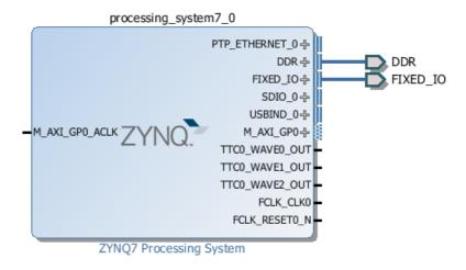
Figure 2.12: Zybo ZYNQ7 Processing System External Connections
