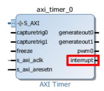
Figure 2.37: AXI Timer in the block design
