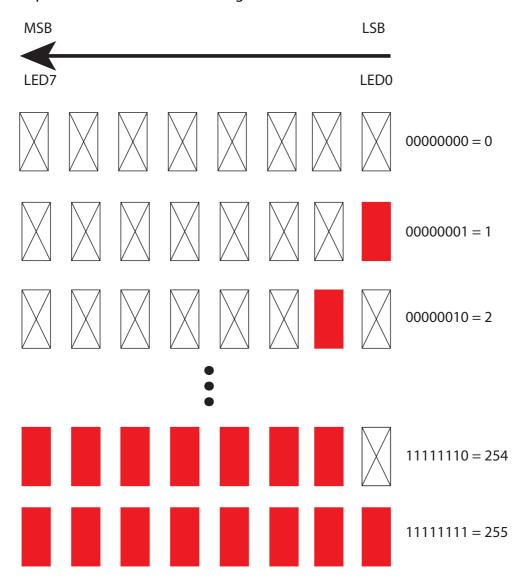
Figure 2.33: Zedboard LED flashing states
