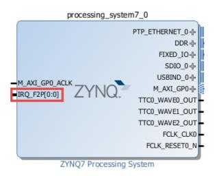
Figure 2.24: Zybo Zynq PS with interrupt port
