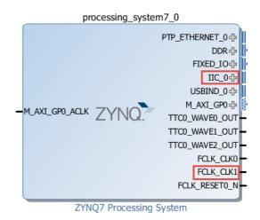
Figure 5.20: Zedboard Zynq7 Processing System block
