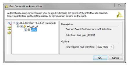
Figure 1.18: Zedboard Run Connection Automation Dialogue - GPIO Block
