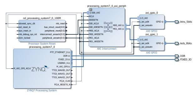
Figure 2.15: Zedboard Zynq Processor System
