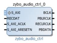
Figure 5.15: Zybo Audio Controller block
