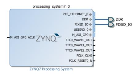
Figure 1.15: Zedboard ZYNQ7 Processing System External Connections
