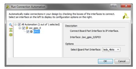
Figure 1.20: Zybo Run Connection Automation Dialogue - GPIO Block
