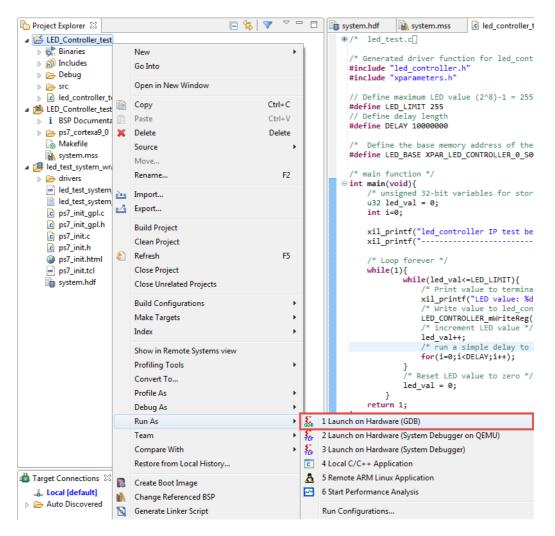
Figure 4.20: Run Application on hardware
