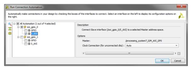
Figure 2.13: Zedboard Run Block Automation - GPIOinstance
