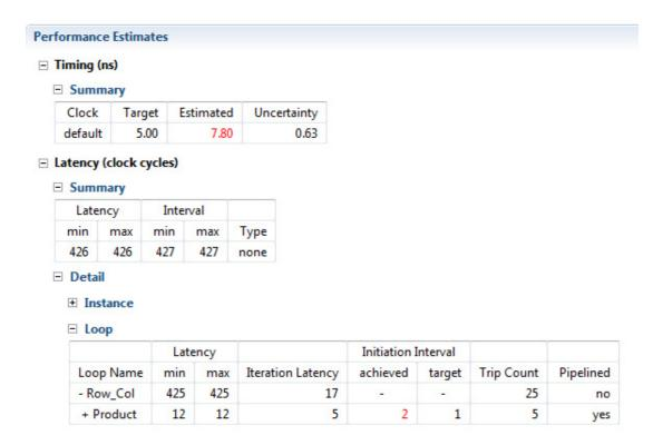
Figure 3.12: Synthesis report for the matrix multiplier, solution2
