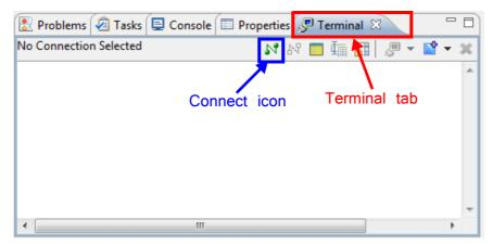
Figure 4.18: SDK Terminal tab
