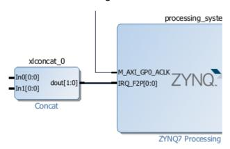
Figure 2.38: Concat in the block design
