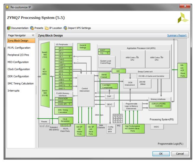
Figure 5.16: Re-customize IP window for Zynq PS
