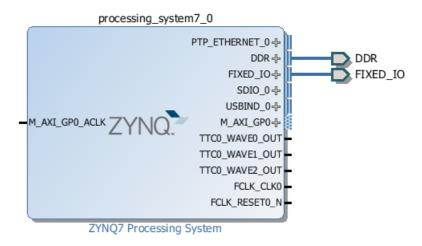
Figure 1.16: Zybo ZYNQ7 Processing System External Connections
