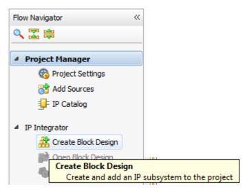
Figure 1.8: Creating a new Block Design in Flow Navigator
