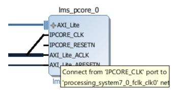
Figure 5.11: Manually connecting the LMS IP CLK
