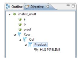
Figure 3.11: Pipelining nested loops in HLS
