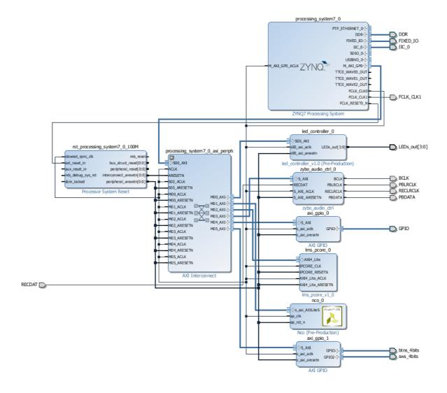
Figure 5.28: Zybo Completed block design
