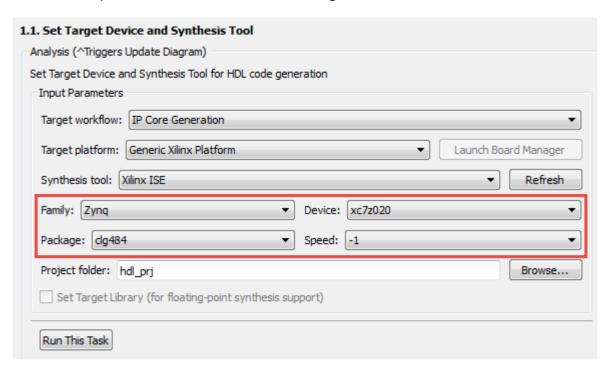
Figure 4.27: ZedBoard HDL Workflow Advisor Input Parameters
