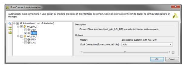
Figure 2.16: Zybo Run Block Automation - GPIOinstance
