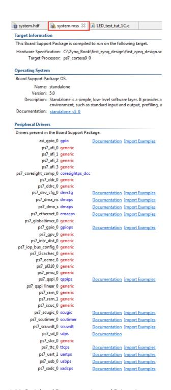
Figure 1.33: Peripheral Documentation and Drivers in system.mss tab
