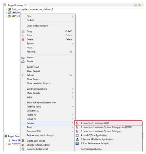
Figure 1.37: Launch Application onto the Zynq Development Board
