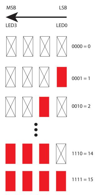
Figure 2.34: Zybo LED flashing states
