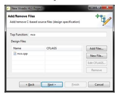
Figure 4.33: Vivado HLS New Project Wizard (Add/Remove Files)
