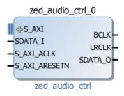
Figure 5.14: ZedBoard Audio Controller block
