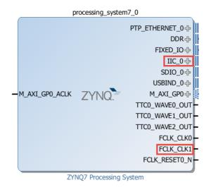
Figure 5.21: Zybo Zynq7 Processing System block
