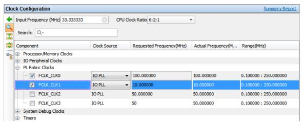
Figure 5.17: Adding a 10 MHz fabric clock
