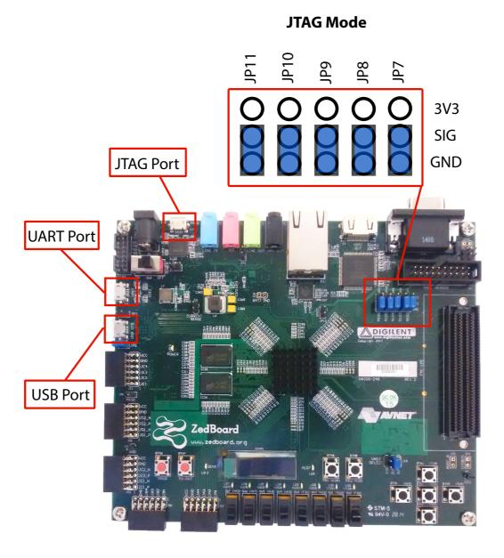
**Figure 1.34:** Zedboard JTAG Jumper Configuration
