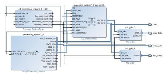
**Figure 2.25:** Zybo Zyng processor system with interrupts
