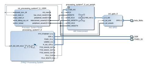
Figure 1.19: Zedboard, Zynq Processor System
