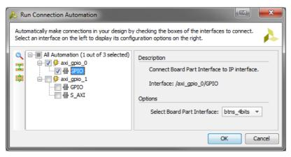
Figure 2.17: Zybo Run Connection Automation dialogue — GPIO
