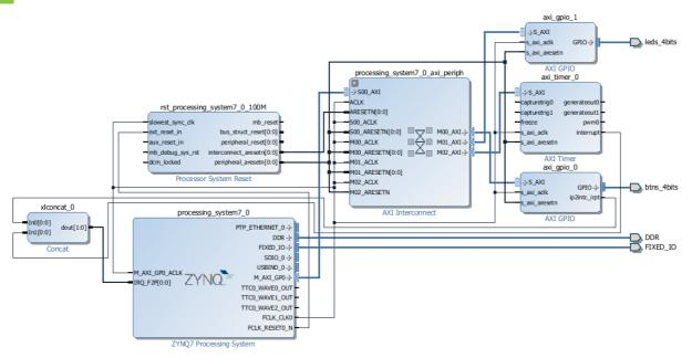
Figure 2.40: Zybo complete system with multiple interrupts sources
