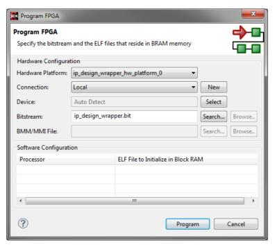
Figure 5.33: Program FPGA window
