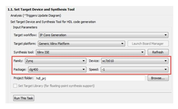
Figure 4.28: Zybo HDL Workflow Advisor Input Parameters
