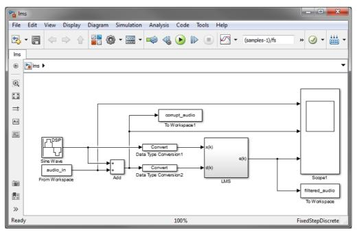
Figure 4.24: LMS model in Simulink
