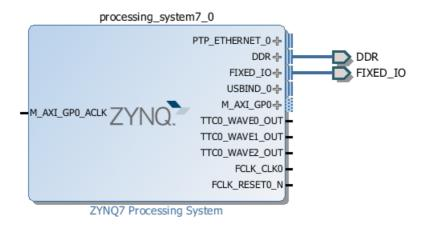
Figure 2.11: Zedboard ZYNQ7 Processing System External Connections
