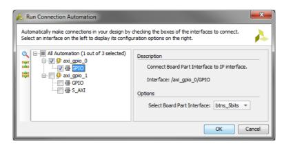
Figure 2.14: Zedboard Run Connection Automation dialogue — GPIO
