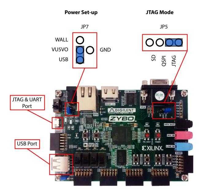
Figure 1.35: Zybo JTAG and Power Jumper Configurations
