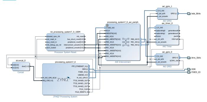
Figure 2.39: Zedboard complete system with multiple interrupts sources
