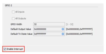
Figure 2.19: Enabling GPIO interrupts
