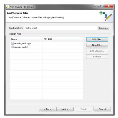
Figure 3.2: Adding files to a Vivado HLS project
