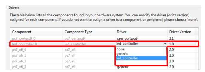
Figure 4.17: LED Controller driver selection
