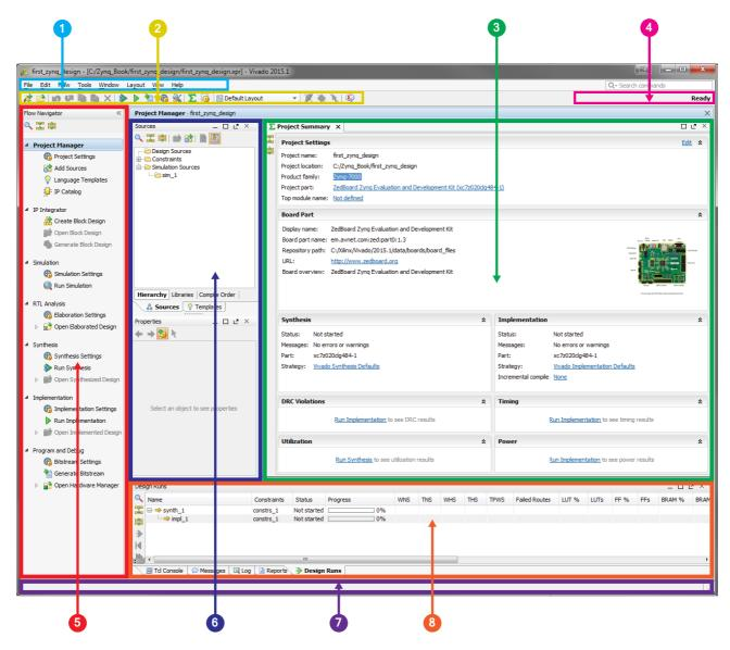
Figure 1.5: Vivado IDE Environment Layout (Zedboard)
