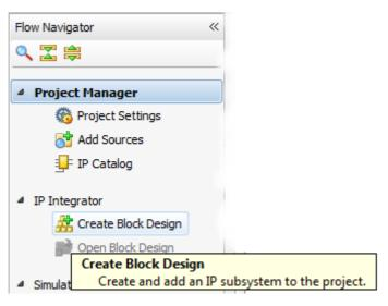
Figure 2.5: Creating a New Block Design in Flow Navigator
