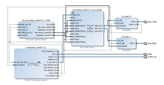
Figure 2.23: Zedboard Zynq processor system with interrupts
