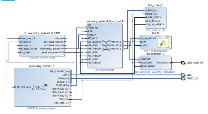
Figure 5.12: Zedboard end of exercise block diagram
