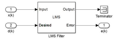
Figure 4.25: LMS subsystem
