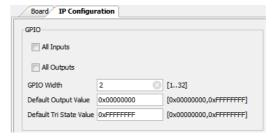
Figure 5.23: Zedboard GPIO width setting
