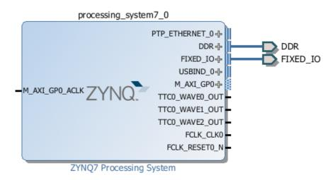
Figure 5.7: Zedboard ZYNQ7 Processing System External Connections
