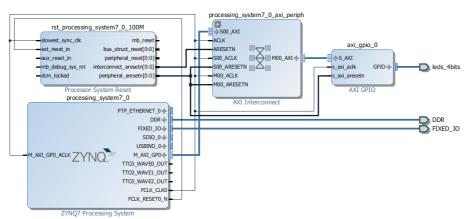
Figure 1.21: Zybo, Zynq Processor System
