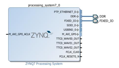
Figure 5.8: Zybo ZYNQ7 Processing System External Connections
