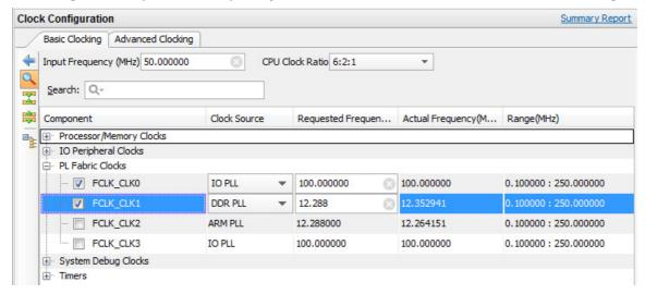
Figure 5.18: Adding a 12.288 MHz fabric clock
