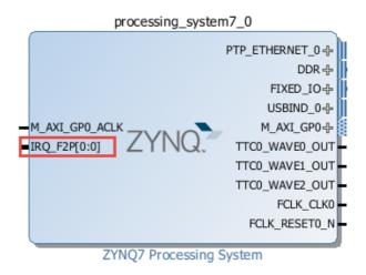
Figure 2.22: Zedboard Zynq PS with interrupt port
