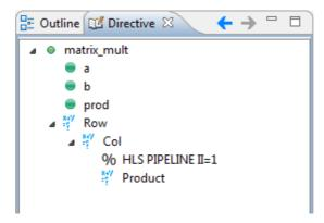
Figure 3.15: Pipelining Column Loop in HLS
