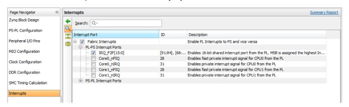
**Figure 2.21:** Configuring Zynq PS to utilise interrupts
