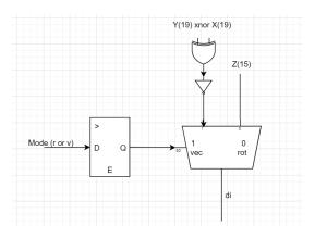
The control diagram above depicts mode selection of the hyperbolic CORDIC based on assignment of input data in the word.
