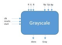
As you can see from the diagram, Grayscale module takes 8 bit R, G, B values, 7 bits Rp, Gp, Bp values. Rp, Gp and Bp are percentage values. These values will be between 0-100 therefore we only need 7bits to represent.
