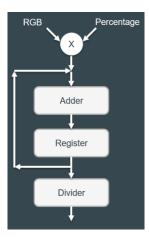
We used Professor Llamocca's multiplier and divider circuits. There were three versions of these circuits; combinatorial, iterative and pipelined. We decided to use fully combinatorial.
