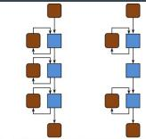
Figure 15. (a) Serial pipeline. Each stage can maintain its state so that later outputs can depend on earlier ones. (b) Parallel pipeline. The parallel stage is stateless; thus, multiple invocations of it can run in parallel.
