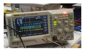
Image 1: Shows the CAN signal reading of transmission in blue and receiver in yellow on an oscilloscope.
