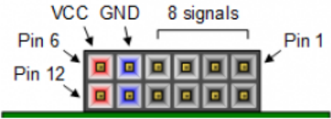
( https://reference.digilentinc.com/_detail/reference/programmable-logic/nexys-a7/n4v.png?id=reference%3Aprogrammable-logic%3Anexys-a7%3Areference-manual ) Figure 10.1 Pmod Connectors; Front View, as Loaded on PCB
