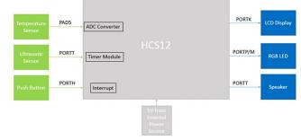
Figure 1. Project Block Diagram
