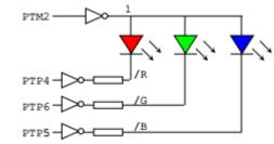
Figure 7: RGB LED diagram showing each PWM port, for RGB respectively this is port 4, 6, and 5.
