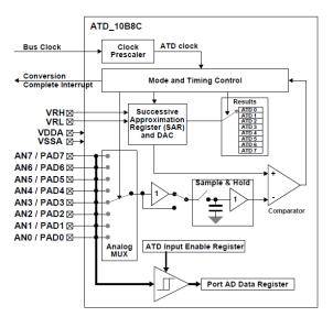
Figure 5. HCS12 ADC Block Diagram
