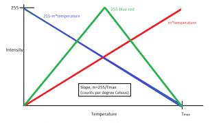
Figure 8: Color scaling vs. temperature
