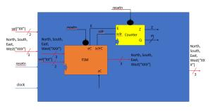
*Block Diagram of Circuit Structure* This unfortunately caused more problems than it solved, so we controlled each one separately. We used the circuit above to allow for a synchronous clock, counter, and fsm, as well as output the lights all together on the proper timing. The counter used was modified based off of the counter provided to us during lab 6 of the semester.
