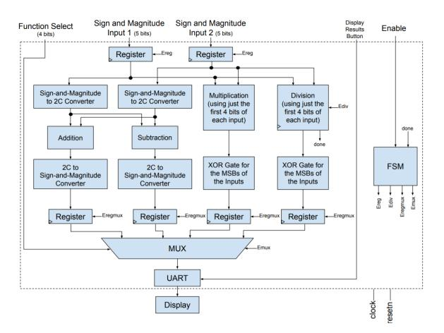
Figure 9: Full Block Diagram of Signed Calculator System
