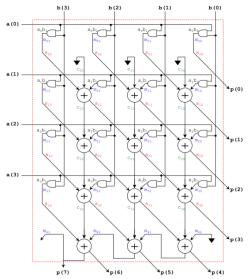
Figure 2: Diagram of 4-bit multiplication
