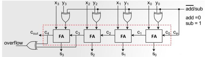
This is a 4-bit adder/sub, and we used a 9-bit adder/ sub
