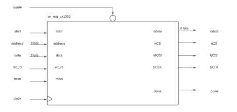
Wr\_reg is made of shift register, primarily, and other components all utilizing a finite state machine to process the data given - 8-bit register with enable
