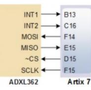
INT1: Interrupt One INT2: Interrupt Two MOSI: Master Out Slave In MISO: Master In Slave Out ~C S: Slave Select (Active Low) SCLK: Serial Clock
