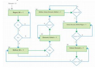
Upon our first implementation of our system on the NEXYs board we noticed that our register was cutting off one bit coming from the PMOD ALS. We fixed this by adjusting the counter reading in the state machine so that it is able to capture all significant bits from the sensor and provide a proper output (0-255) on the seven segment today.
