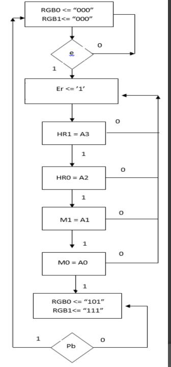
←2<sup>nd</sup> Finite State Machine: Alarm portion of Alarm Clock
