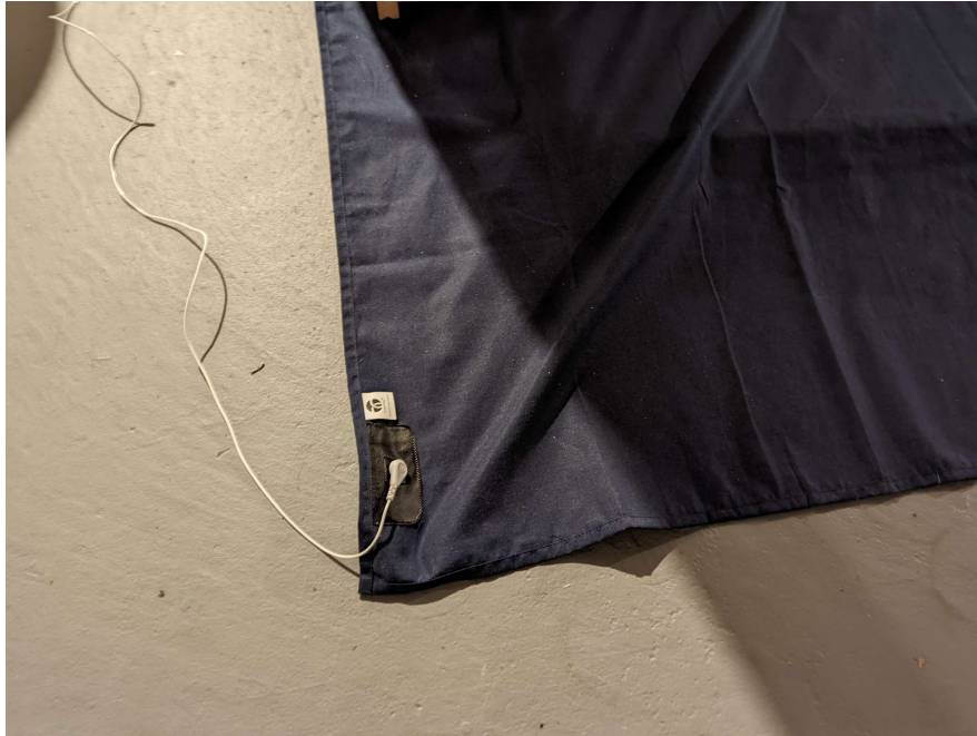
Figure 6. Detail of the wired grounding mat placed on the floor underneath the experiment area.
