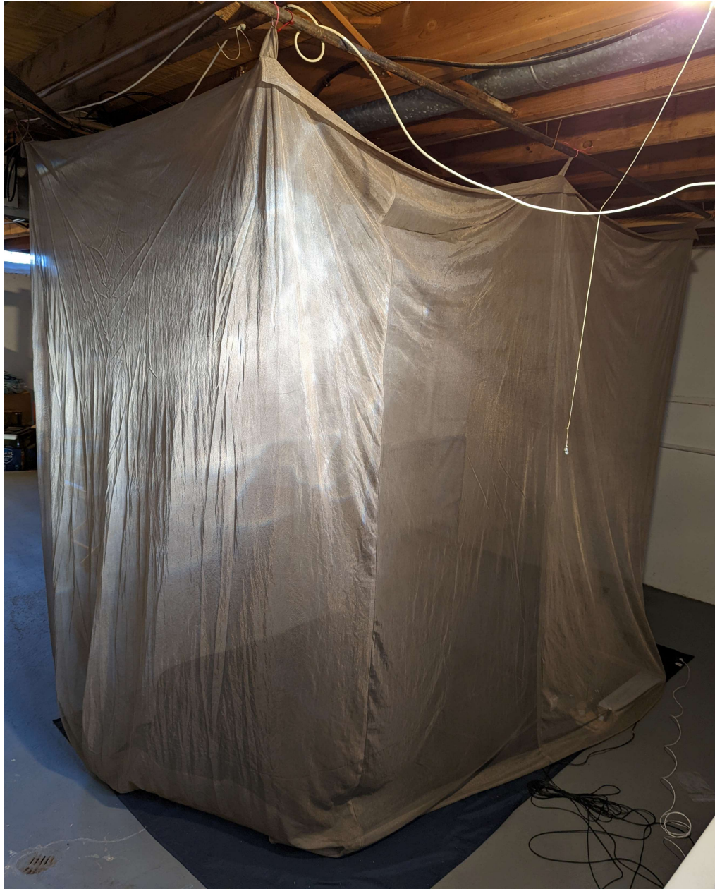
Figure 5. RF signal shield setup.
