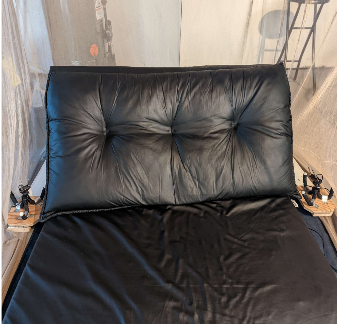
Figure 9. The setup for human subject data acquisition inside the shield. Two SDR devices were fixed on either side of the human subject and pointing to the human subject.
