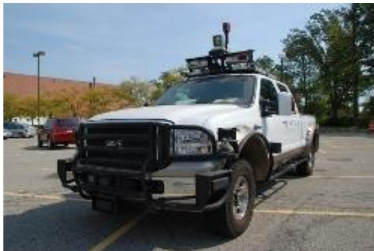
Figure 4.16: The device for outdoor mapping [9].
