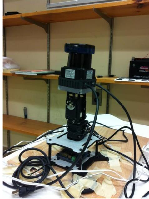
Figure 2.2: Turret Widow X servo (left); LiDAR with Turret Widow X servo (right).
