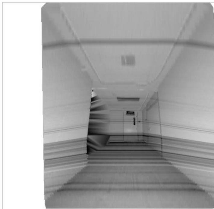
Figure 4.6: Generation of LiDAR 2D intensity image for location 1.
