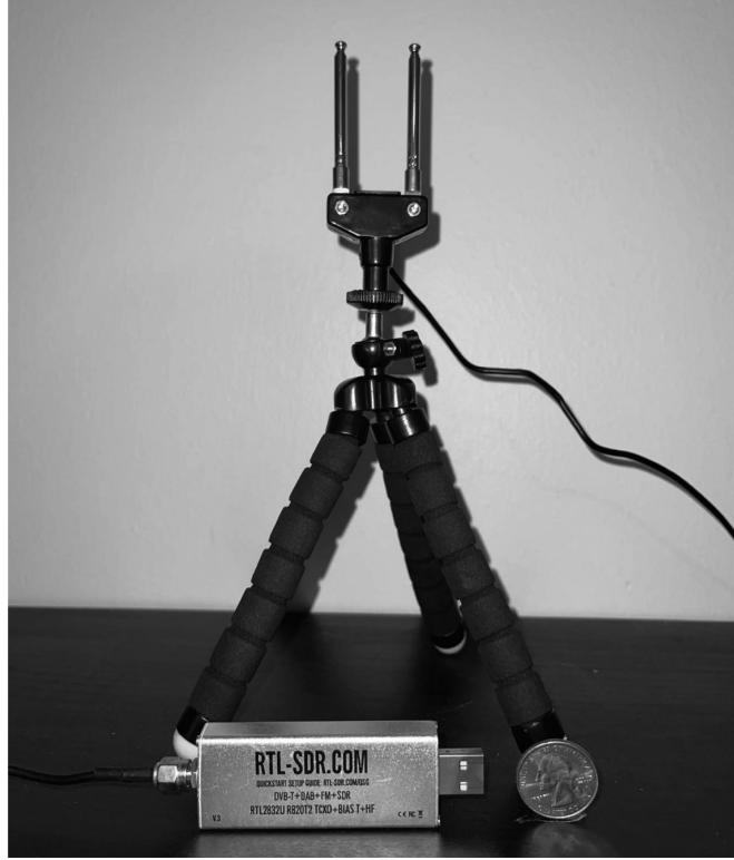
Fig. 2. RTL-SDR RTL2832U is used as PRF sensor to collect PRF spectrum.
