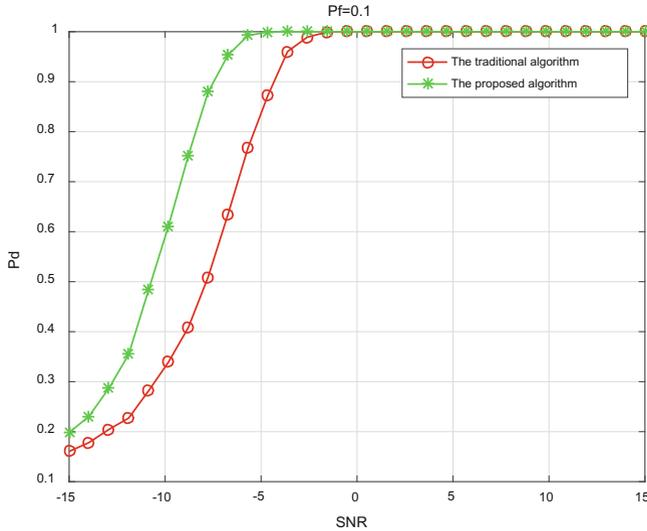
Fig. 4. The detection probability versus SNR at  $P_{fd} = 0.1$ .
