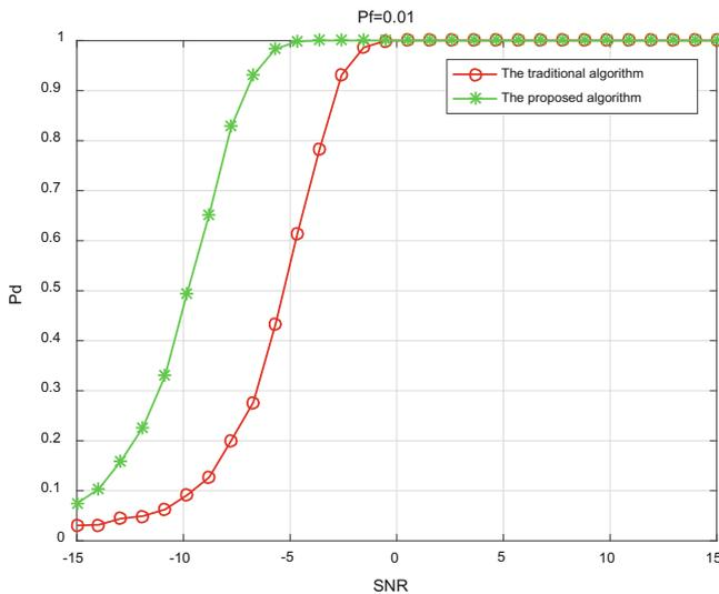
Fig. 5. The detection probability versus SNR at  $P_{fd} = 0.01$ .
