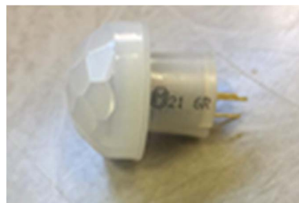
Fig. 1. Panasonic AMN24112 PIR sensor with analog output capability.
