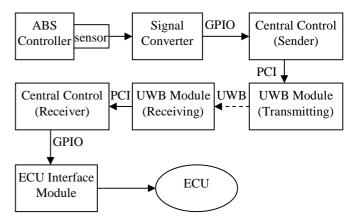
Figure 2. Testbed components and data flow
