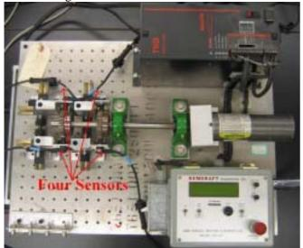
Figure 3. ABS motor control simulating system and wheel speed sensors
