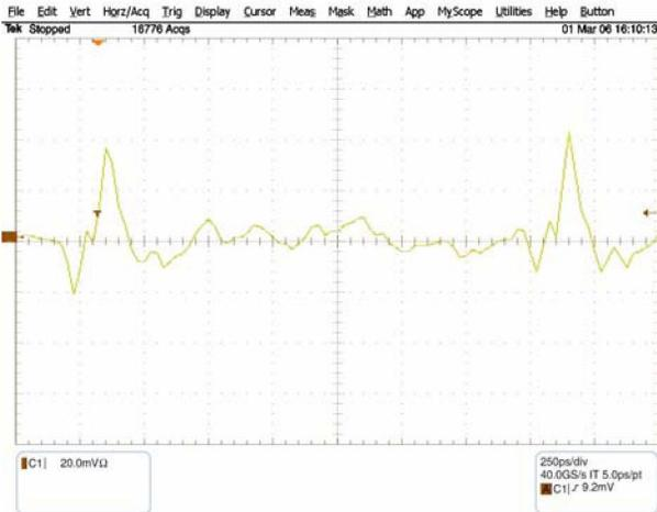
Fig. 7 The received signal in the Experiment 1 within the engine compartment. A line-of-site exists between antennas.
