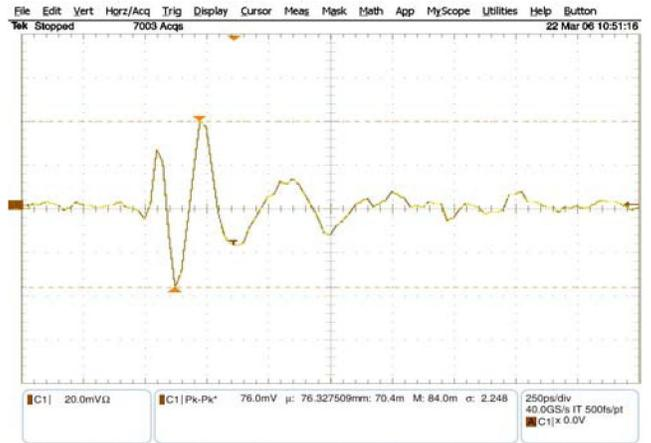
Fig. 5 The received signal at the antenna under the engine compartment. The transmitting antenna was positioned on the rear left wheel.
