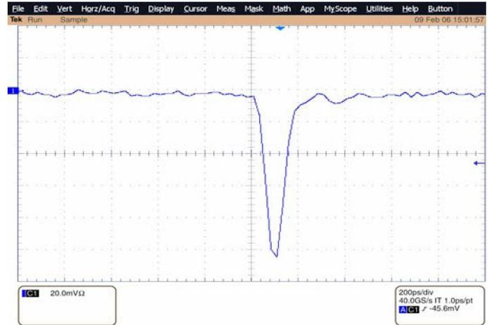
Fig. 2 The UWB pulse at the Pulse Generator output.
