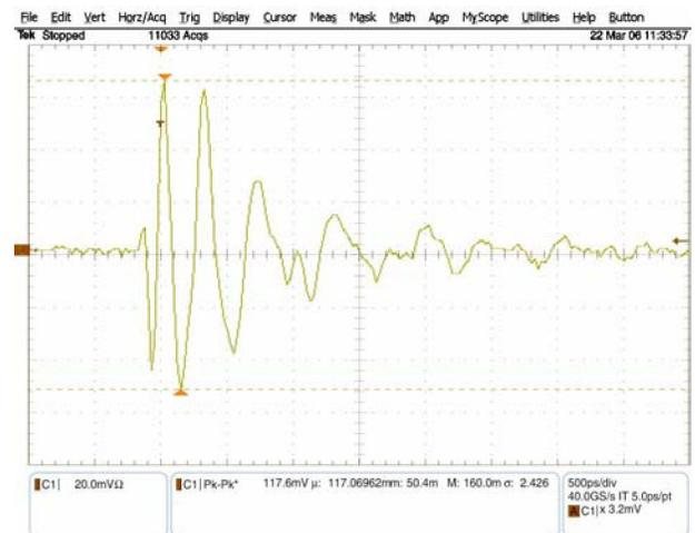
Fig. 6 The received signal at the antenna under the engine compartment. The transmitting antenna was positioned on the rear right wheel.
