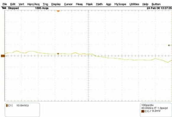
Fig. 4 The received noise when the transmitter was turned off.
