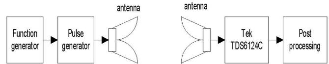
Fig. 1 Block diagram of the UWB channel sounding setup.
