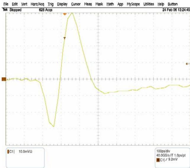
Fig. 3 The received signal in a lab. The transmitting antenna and the receiving antenna were 211 inches away from each other at the height of 44 inches.
