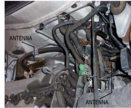
Fig. 8 The UWB Experiment 2 within the engine compartment. Antennas were installed deep in the engine compartment. A large piece of metal shield blocked antennas from seeing each other. There was no line-of-sight. The curve is the received signal. The picture is the experiment setup.
