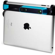
Figure 8: Portable 3D sensor mounted on iPad
