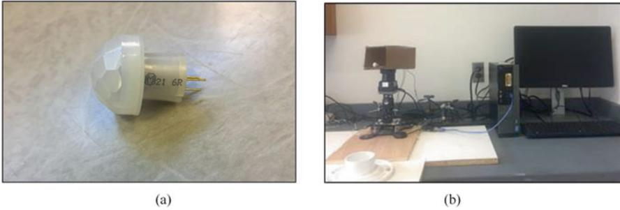
**Fig. 1** Novel MI-PIR system including the (a) the Panasonic AMN24112 and (b) the full design
