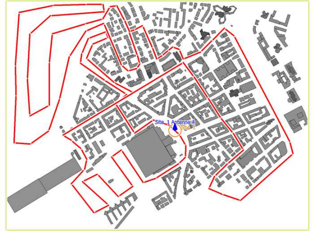
Figure 2. Urban canyon scenario with base station located in center of city at a height of 80 meters.
