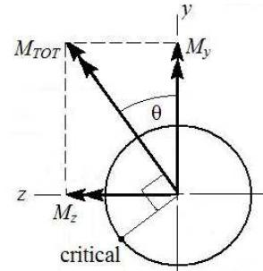
The combined bending moment vector is at an angle of 30.3° CCW from the y axis. The critical bending stress location will be 90° CCW from this vector, where the tensile bending stress is additive with the tensile axial stress. The critical stress element is therefore on the outer surface, at an angle of 30.3° CCW from the z axis.
