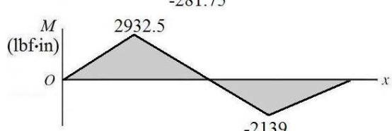
**(d)** The maximum bending moment is at  $x = 10$  in, and is  $M = 2932.5$  lbf-in. Since the shaft rotates, each stress element will experience both positive and negative bending stress as it moves from tension to compression. The torque transmitted through the shaft
