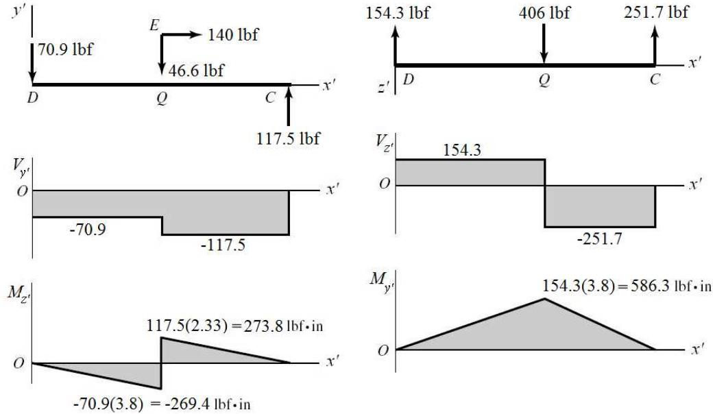
(c) The critical stress element is just to the right of  $Q$ , where the bending moment in both planes is a maximum, and where the torsional and axial loads exist.
