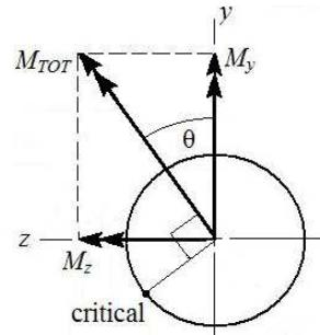
The combined bending moment vector is at an angle of 37.4° CCW from the y axis. The critical bending stress location will be 90° CCW from this vector, where the tensile bending stress is additive with the tensile axial stress. The critical stress element is therefore on the outer surface, at an angle of 37.4° CCW from the z axis.
