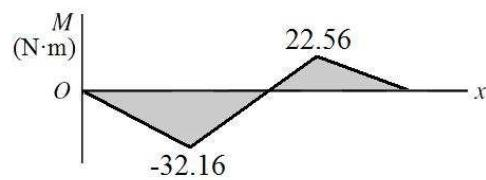
**(d)** From the bending moment diagrams, it is clear that the critical location is at A where both planes have the maximum bending moment. Combining the bending moments from the two planes,
