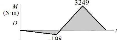
(d) From the bending moment diagrams, it is clear that the critical location is at B where both planes have the maximum bending moment. Combining the bending moments from the two planes,
