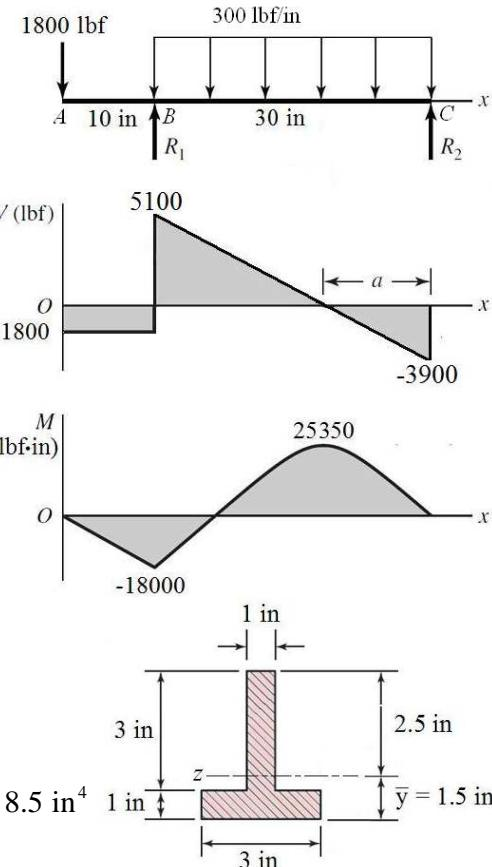
the transverse shear is maximum, or (iii) in the web just above the flange where bending stress and shear stress are in their largest combination.
