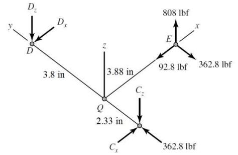
(b) For  $DQC$ , let  $x', y', z'$  correspond to the original  $-y, x, z$  axes.
