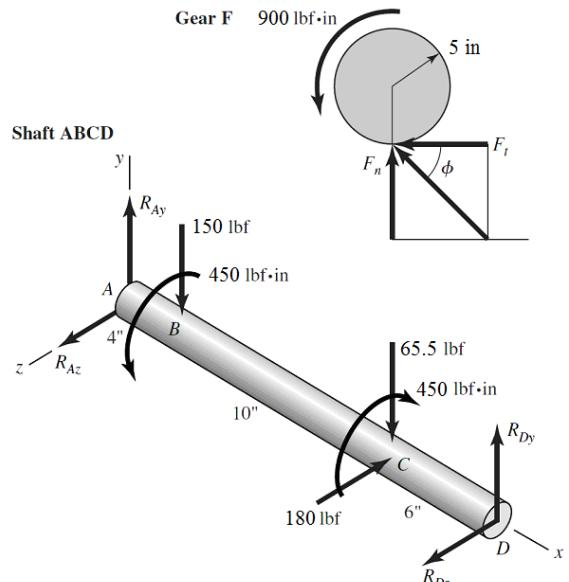
$$\sum(M_A)_z = 0 = 20R_{Dy} - 65.5(14) - 150(4) \Rightarrow R_{Dy} = 75.9 \text{ lbf}$$
