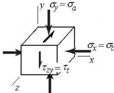
(d) Analyze the stress element from part (c) using the equations developed in parts (a) and (b).
