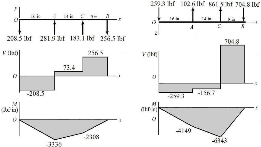
(d) Combine the bending moments from both planes at A and C to find the critical location.
