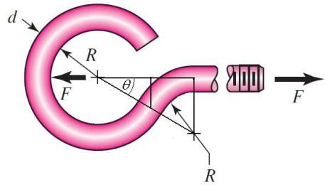
Using Eq. (3-65) for the bending stress, and combining with the axial stress,
