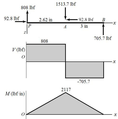
**(c)** The critical stress element is just to the left of A, where the bending moment in both planes is a maximum, and where the torsional and axial loads exist.
