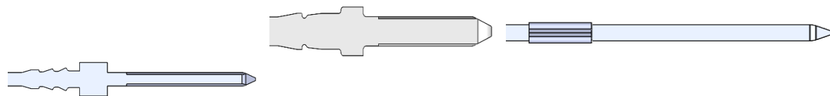
Three main retention features: Tree shape (left), barbed (middle), and bandolier (right)
