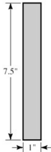
*Material properties:* The allowable stress given is low. Let's demonstrate that. For the 1020 CD bracket, use HR properties of  $S_y = 30$  kpsi and  $S_{ut} = 55$ . The 1030 HR support,  $S_y = 37.5$  kpsi and  $S_{ut} = 68$ . The E6010 electrode has strengths of  $S_y = 50$  and  $S_{ut} = 62$  kpsi.
