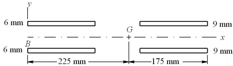
For the pattern in bending shown, find the centroid  $G$  of the weld group.
