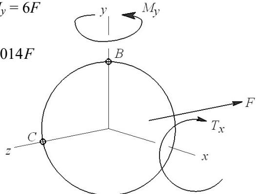
C: Direct shear, torsion, and bending.
