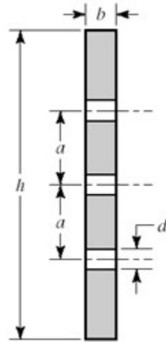
Failure is predicted for bolt shear and bearing on member.
