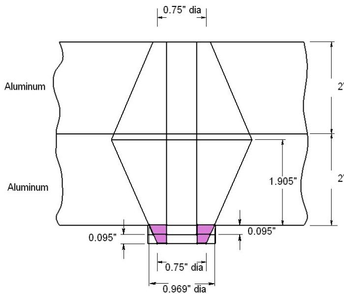
Upper aluminum frustum:  $t = [4 + 2(0.095)]/2 = 2.095 \text{ in}$ ,  $d = 0.5 \text{ in}$ ,  $D = 0.75 \text{ in}$ , and  $E = 10.3 \text{ Mpsi}$ . From Eq. (8-20)
