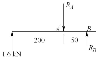
$$\begin{aligned}\sum M_B &= 0 & 1.6(250) - 50R_A &= 0 \Rightarrow R_A = 8 \text{ kN} \\ \sum M_A &= 0 & 200(1.6) - 50R_B &= 0 \Rightarrow R_B = 6.4 \text{ kN}\end{aligned}$$
