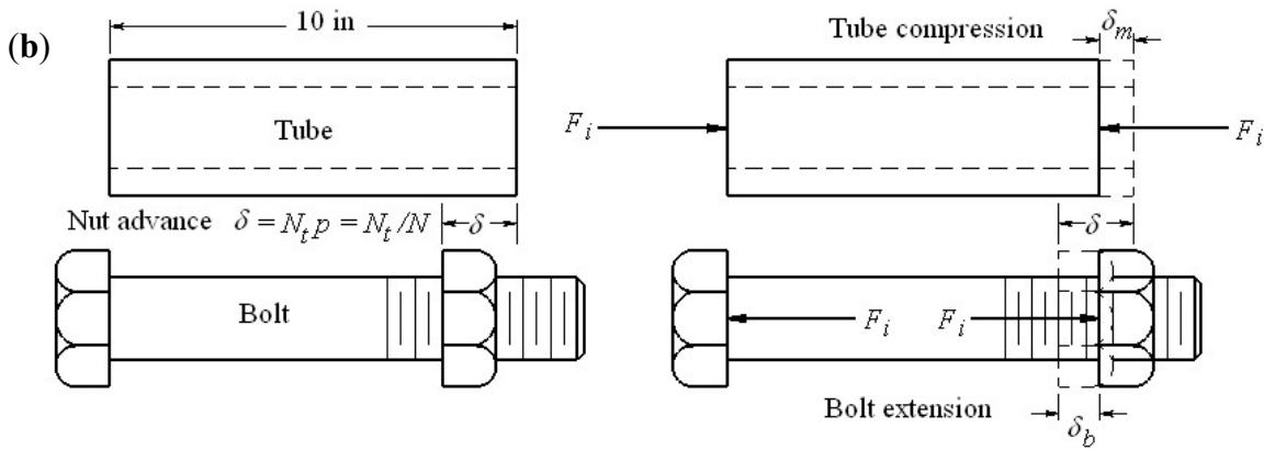
Let:  $N_t$  = no. of turns,  $p$  = pitch of thread (in),  $N$  = no. of threads per in =  $1/p$ . Then,
