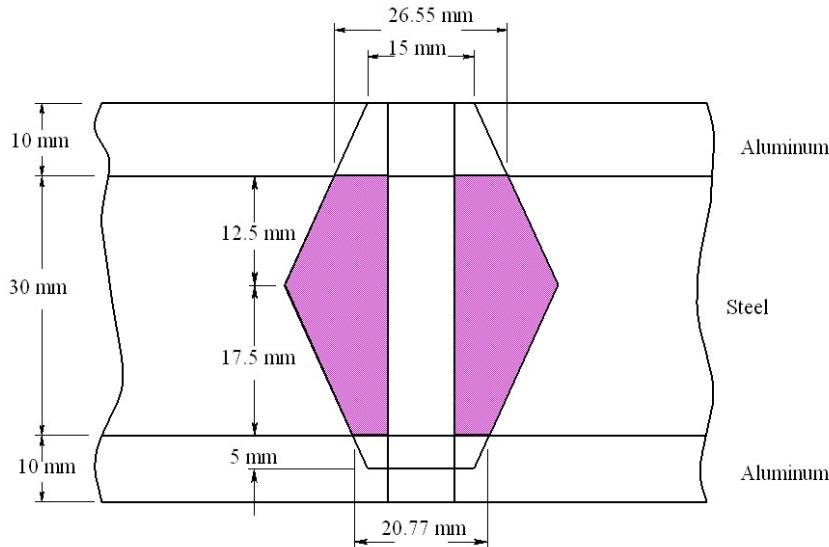
Upper aluminum frustum:  $t = 10 \text{ mm}$ ,  $d = 10 \text{ mm}$ ,  $D = 15 \text{ mm}$ , and  $E = 71 \text{ GPa}$ . From Eq. (8-20)
