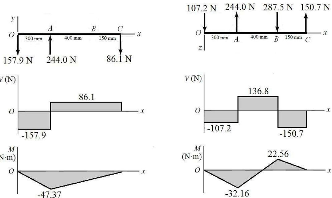
(d) From the bending moment diagrams, it is clear that the critical location is at A where both planes have the maximum bending moment. Combining the bending moments from the two planes,
