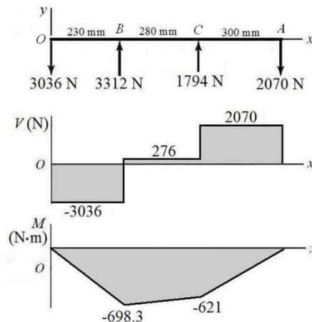
(d) The maximum bending moment is at  $x = 230$  mm, and is  $M = -698.3$  N·m. Since the shaft rotates, each stress element will experience both positive and negative bending stress as it moves from tension to compression. The torque transmitted through the shaft from  $A$  to  $B$  is  $T = (1800 - 270)(0.200) = 306$  N·m. For a stress element on the outer surface where the bending stress and the torsional stress are both maximum,
