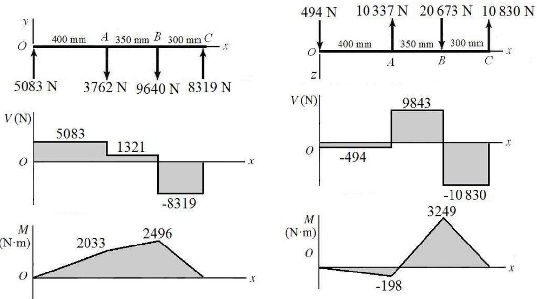
(d) From the bending moment diagrams, it is clear that the critical location is at B where both planes have the maximum bending moment. Combining the bending moments from the two planes,
