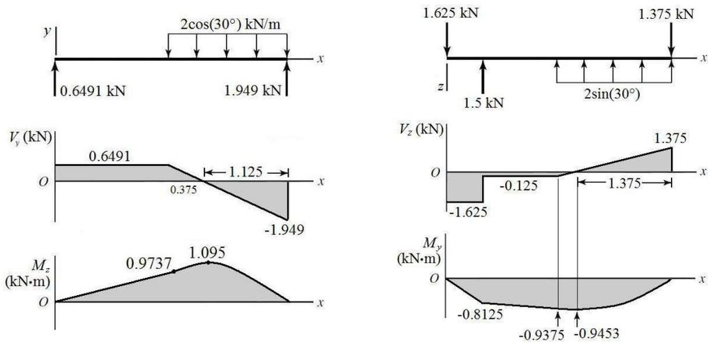
(c) The transverse shear and bending moments for most points of interest can readily be taken straight from the diagrams. For  $1.5 < x < 3$ , the bending moment equations are parabolic, and are obtained by integrating the linear expressions for shear. For convenience, use a coordinate shift of  $x' = x - 1.5$ . Then, for  $0 < x' < 1.5$ ,
