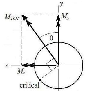
The combined bending moment vector is at an angle of  $30.3^\circ$  CCW from the *y* axis. The critical bending stress location will be  $90^\circ$  CCW from this vector, where the tensile bending stress is additive with the tensile axial stress. The critical stress element is therefore on the outer surface, at an angle of  $30.3^\circ$  CCW from the *z* axis.
