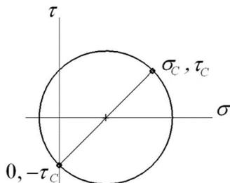
$$\begin{aligned} \tau_{\max} &= \sqrt{\left(\frac{\sigma_C}{2}\right)^2 + \tau_C^2} \\ &= \sqrt{\left(\frac{9.60}{2}\right)^2 + 0.9^2} = 4.88 \text{ MPa} \quad \text{Ans.} \end{aligned}$$
