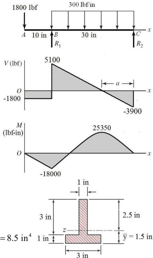
$x = 27$  in: (i) at the top where the bending stress is maximum, (ii) at the neutral axis where the transverse shear is maximum, or (iii) in the web just above the flange where bending stress and shear stress are in their largest combination.
