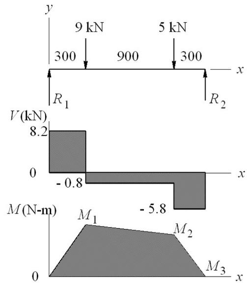
$$\begin{aligned} M_1 &= 8.2(300) = 2460 \text{ N} \cdot \text{m} \quad \text{Ans.} \\ M_2 &= 2460 - 0.8(900) = 1740 \text{ N} \cdot \text{m} \quad \text{Ans.} \\ M_3 &= 1740 - 5.8(300) = 0 \quad \text{checks!} \end{aligned}$$
