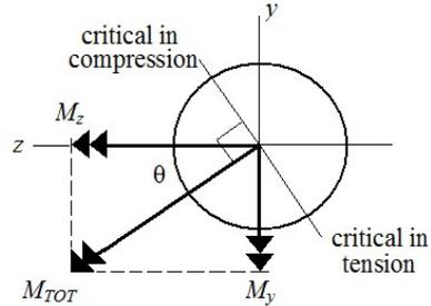
The combined bending moment vector is at an angle of  $29.7^\circ$  CCW from the  $z$  axis. The critical bending stress location, and thus the critical stress element, will be  $\pm 90^\circ$  from this vector, as shown. There are two equally critical stress elements, one in tension ( $119.7^\circ$  CCW from the  $z$  axis) and the other in compression ( $60.3^\circ$  CW from the  $z$  axis). We'll continue the analysis with the element in tension.
