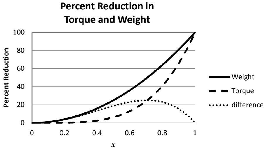
The value of greatest difference in percent reduction of weight and torque is 25% and occurs at  $x = \sqrt{2}/2$ .
