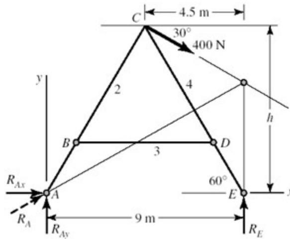
Step 2: Find components of  $R_C$  and  $R_D$  on link 4
