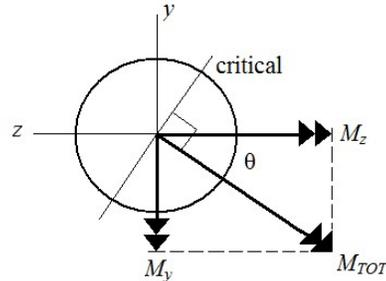
The combined bending moment vector is at an angle of  $36.3^\circ$  CW from the negative  $z$  axis. The critical bending stress location will be  $\pm 90^\circ$  from this vector, as shown. Since there is an axial stress in tension, the critical stress element will be where the bending is also in tension. The critical stress element is therefore on the outer surface at the wall, at an angle of  $36.3^\circ$  CW from the  $y$  axis.
