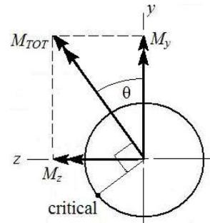
The combined bending moment vector is at an angle of  $37.4^\circ$  CCW from the  $y$  axis. The critical bending stress location will be  $90^\circ$  CCW from this vector, where the tensile bending stress is additive with the tensile axial stress. The critical stress element is therefore on the outer surface, at an angle of  $37.4^\circ$  CCW from the  $z$  axis.
