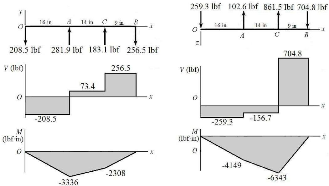
(d) Combine the bending moments from both planes at A and C to find the critical location.
