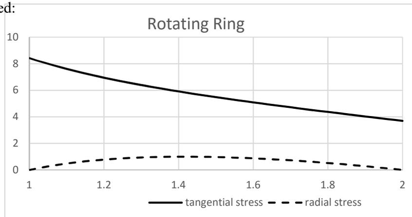
**(b)** The tangential stress,  $\sigma_t$  is maximum at  $r = r_i$  and is given by
