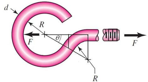
Using Eq. (3-65) for the bending stress, and combining with the axial stress,
