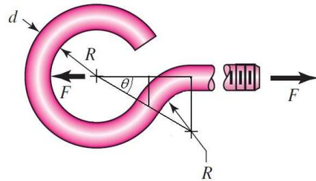
**3-138**  $d = 0.25 \text{ in}$ ,  $r_i = 0.5 \text{ in}$ ,  $r_o = 0.75 \text{ in}$
