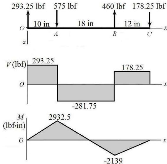
**(d)** The maximum bending moment is at  $x = 10$  in, and is  $M = 2932.5$  lbf·in. Since the shaft rotates, each stress element will experience both positive and negative bending stress as it moves from tension to compression. The torque transmitted through the shaft
