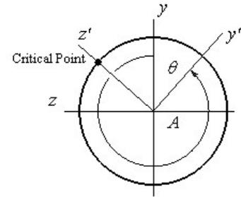
(b)  $\sigma_{\text{bend}} = \frac{|M|c}{I} = \frac{32|M|}{\pi d^3} = \frac{32(1869)}{\pi(0.75^3)} 10^{-3} = 45.13 \text{ kpsi}$
