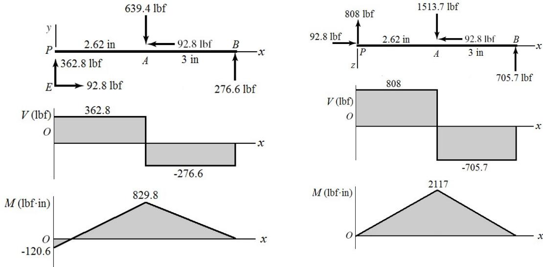
(c) The critical stress element is just to the left of  $A$ , where the bending moment in both planes is a maximum, and where the torsional and axial loads exist.
