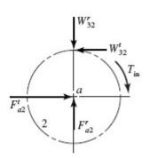
Each bearing on shaft a has the same radial load of  $R_A = R_B = 662/2 = 331$  lbf.
