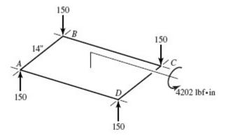
The compressive loads at A and D are absorbed by the base plate, not the bolts. For  $W_{32}^t$ , the tensions in C and D are
