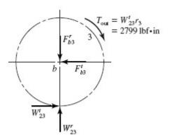
Each bearing on shaft b has the same radial load which is equal to the radial load of bearings A and B. Thus, all four bearings have the same radial load of 331 lbf. Ans.
