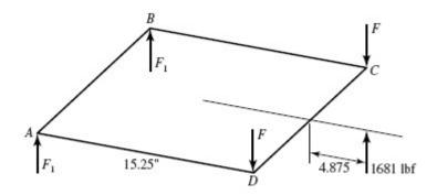
If  $W_{32}^t$  reverses, 15.25 in changes to 13.25 in, 4.815 in changes to 2.875 in, and the forces change direction. For A and B,
