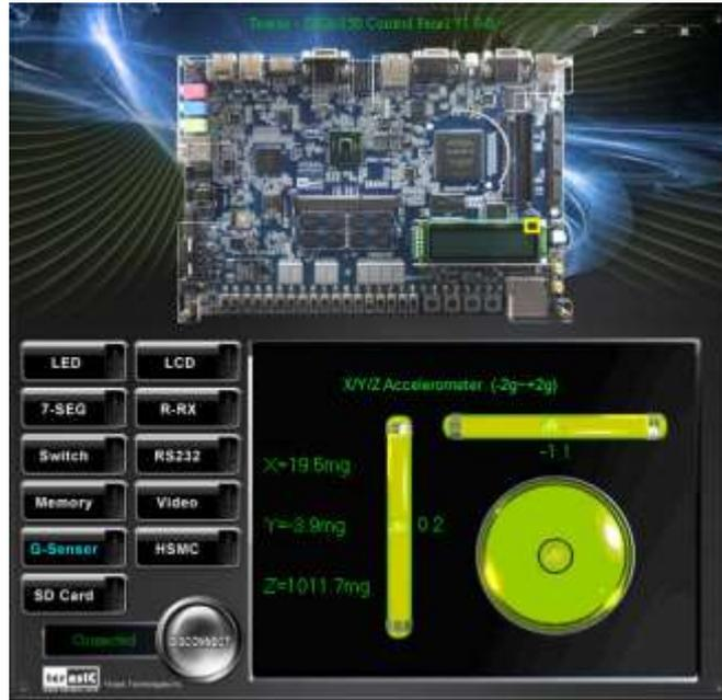
Figure 2-13 Testing the G-sensor
