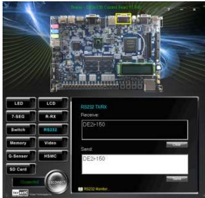
Figure 2-9 RS-232 Serial Communication
