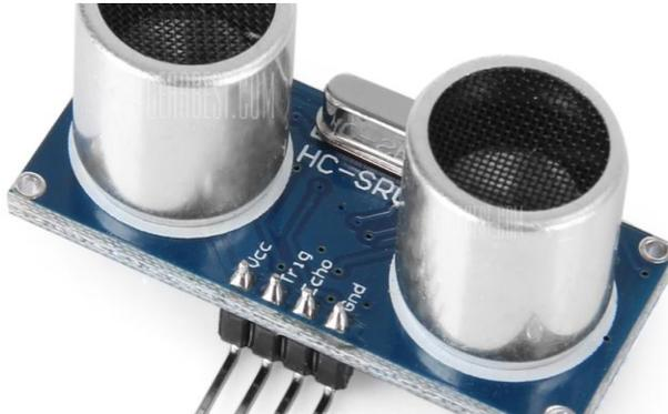
**Figure 3: Sonar Sensor Model HC-SR04**
