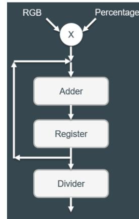
We used Professor Llamocca's multiplier and divider circuits. There were three versions of these circuits; combinatorial, iterative and pipelined. We decided to use fully combinatorial.
