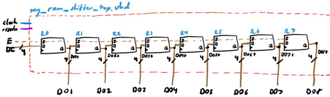
Figure 2. RAM Shift Register Block Diagram
