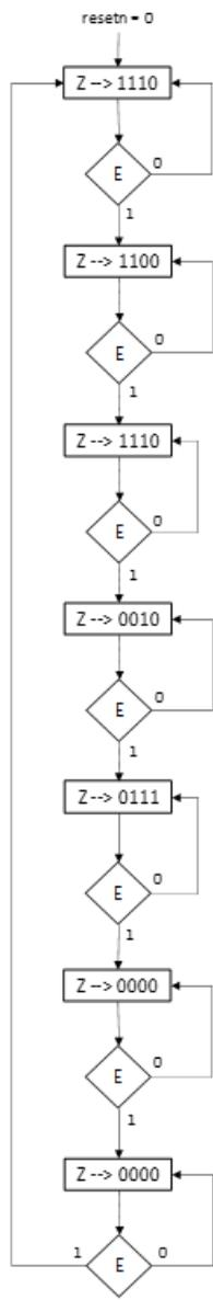
Figure 3. RAM Shift Register FSM State Diagram
