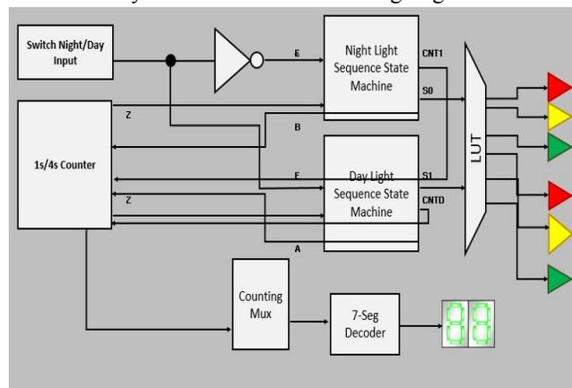
determine the mode of the lights, the command is sent to two different finite state machines that take that input and the output of multiple counters and determines the desired output needed to control the counter and the LEDs.
