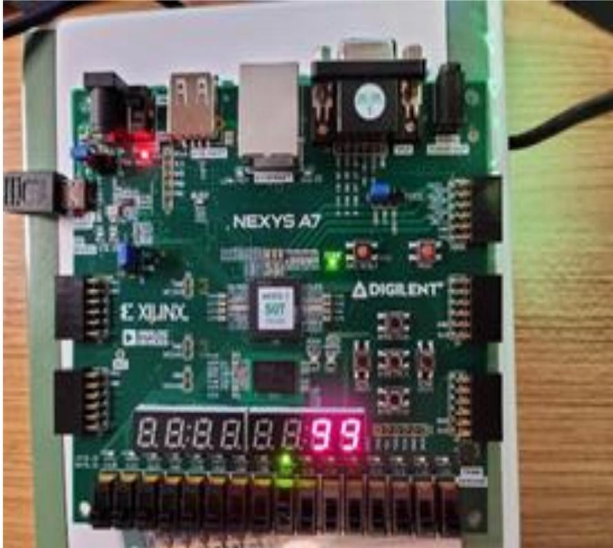
Our system is designed to be able to count to a maximum number of 99 vehicles. When BCD count reaches 99, we only allow cars to exit. For those reasons, the gate in will be closed although sensor A is activated, and only the gate out can be opened when sensor B is activated.
