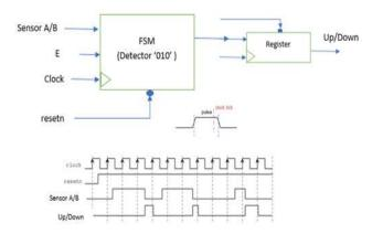
When sensors do not detect any cars entering or exiting the parking garage, they will signal active low '0', and will signal Active high when cars enter or exit. However, when cars rarely move in or out, the sensor will go back '0'. The FSM detector "010" will be used in VHDL code to detect cars in or out, and it will output Up and output Down of the FSMs to connect BCD U/D Counter.
