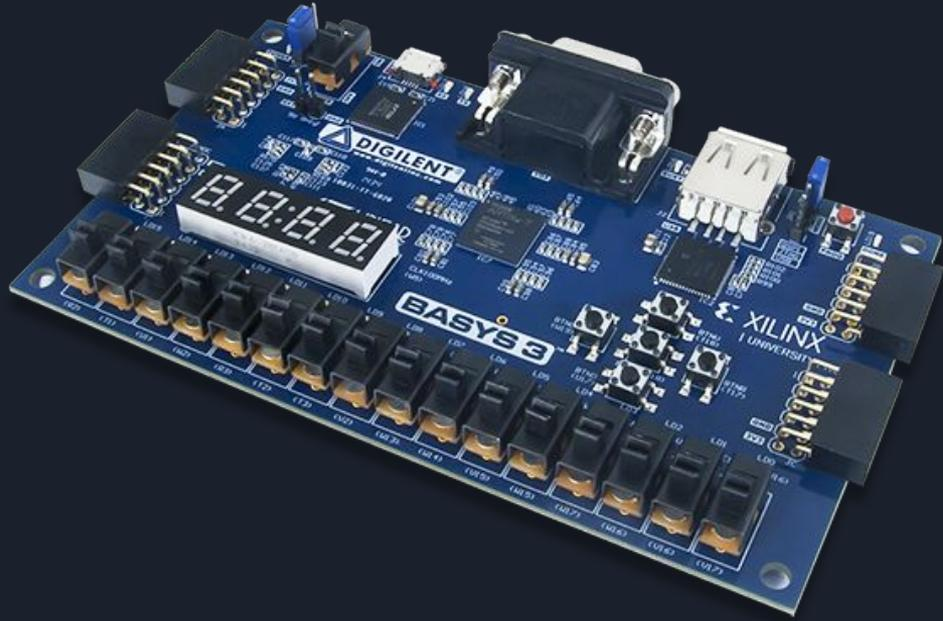
The main purpose of this project is to build and design a circuit that will interface ALL eight segment displays onto the Basys 3 Artix-7 FPGA Trainer Board
