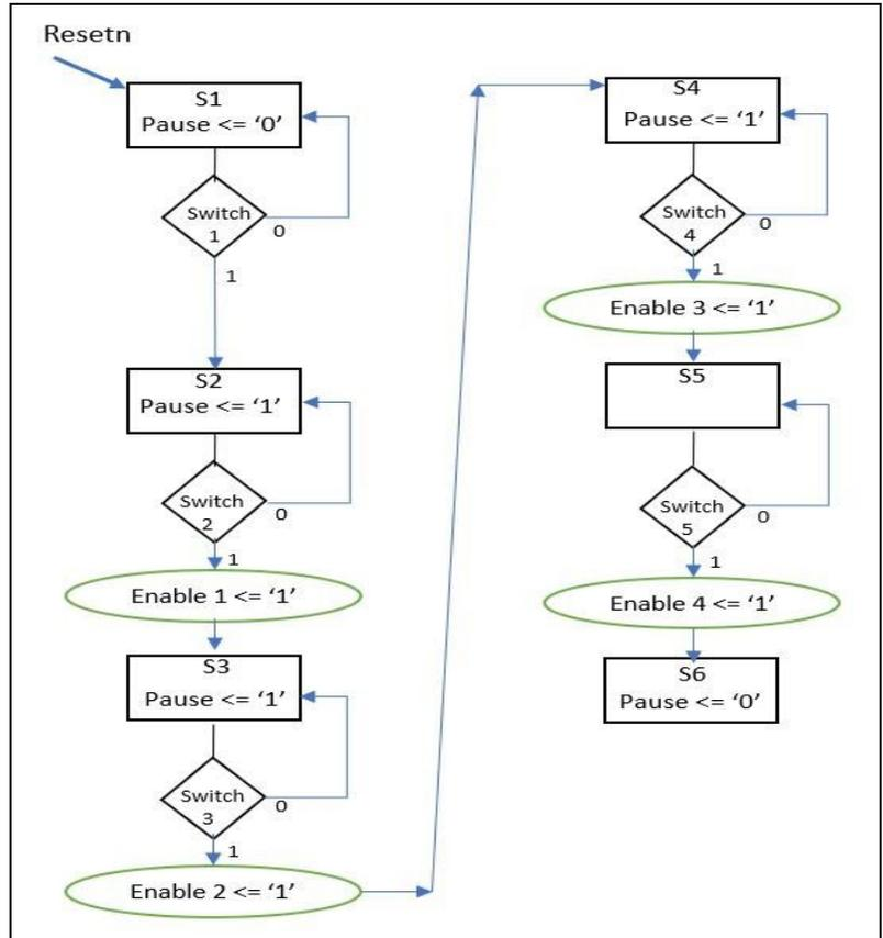
FSM 2 (see below) is slightly more complex as it is required to start the timer when the first light beam is broken, and enable the appropriate row of registers to record the lap times as the next sensors are triggered. When the last sensor is tripped, it stops the timer, and the times can be viewed on the display based on the user's selection. The flow diagram below shows FSM 2.
