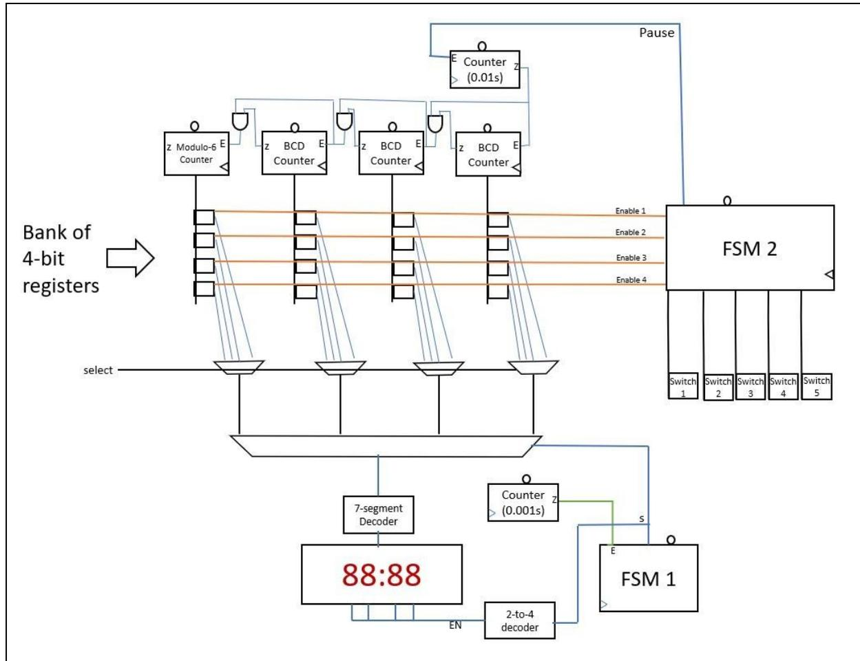
Basically it is composed of a series of counters to keep time, Registers to store lap times, and the appropriate architecture to display the times on the 7 segment display.
