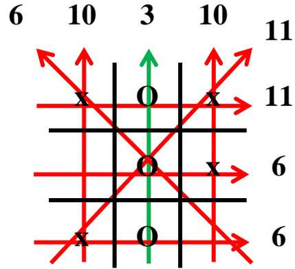
of ‘3’ indicates an ‘O’ win. For each win combination the system combines two 4-bit adders to add three of the registers, and then uses two comparators to test if they sum to ‘15’ or ‘3’. Each of the 8 combinations is tested and if any or multiple result in a win the game halts and a win signal is output. If no player has won a “no win” signal allows players to keep placing moves in memory.
