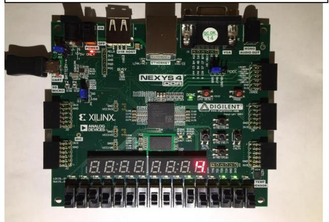
DataA = 6 by SW(0-3) , DataB = 2 by SW(4-7), LEDs indicate the switch is on, subtraction mode enabled by SW(13). Provides the output on the 7-segment display which is  $6-2=4$ .
