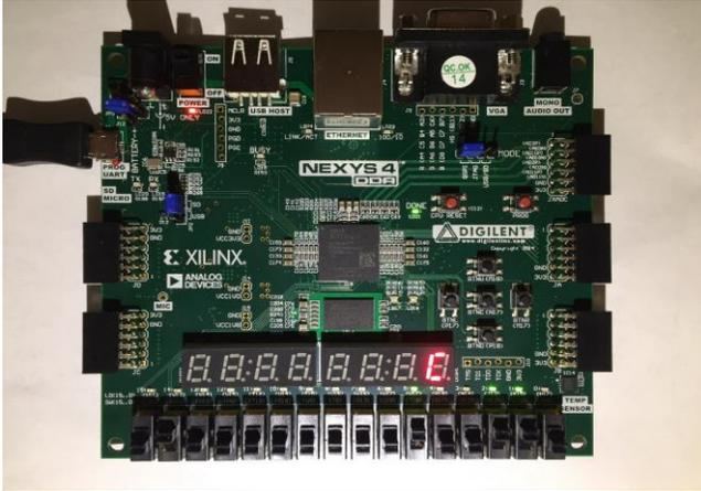
DataA = 6 by SW(0-3) , DataB = 2 by SW(4-7), LEDs indicate the switch is on, multiplication mode enabled by SW(14). Provides the output on the 7-segment display which is  $6*2=C$  or 12.
