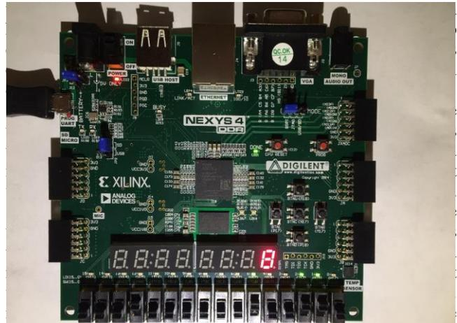
DataA = 6 by SW(0-3) , DataB = 2 by SW(4-7), LEDs indicate the switch is on, addition mode enabled by SW(12). Provides the output on the 7-segment display which is  $6+2=8$ .
