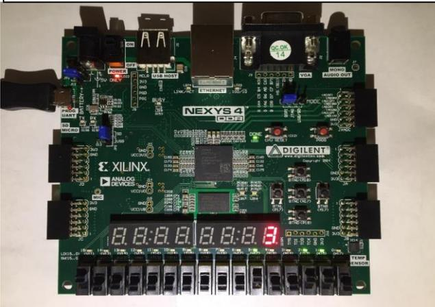
DataA = 6 by SW(0-3) , DataB = 2 by SW(4-7), LEDs indicate the switch is on, division mode enabled by SW(15). Provides the output on the 7-segment display which is  $6/2=3$ .
