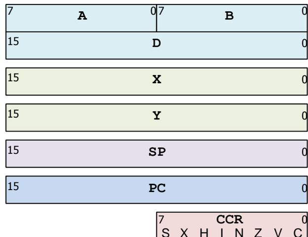
An HCS12 microcontroller also includes I/O registers, subdivided into: data, data direction, control, and status registers. They occupy the memory space (or address space).
