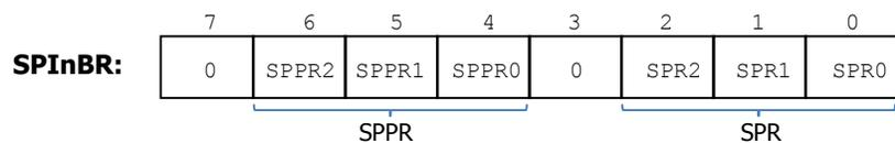
$$\text{Baud Rate} = \frac{E - \text{clock}}{\text{Baud Rate Divisor}}, \text{Baud Rate Divisor} = (\text{SPPR} + 1) \times 2^{(\text{SPR} + 1)}$$
