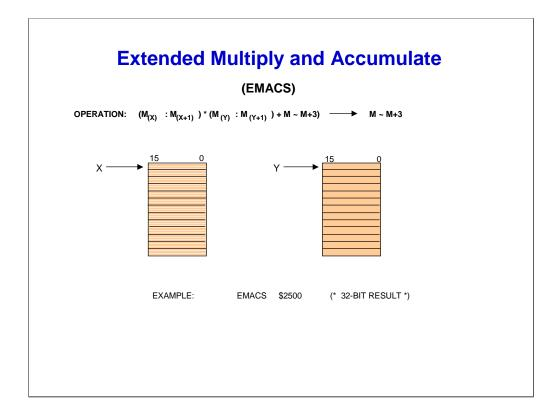
Extended Multiply and Accumulate (EMACS) Instruction allows for multiply and accumulate operations by multiplying two 16-bit operands to produce a 32-bit intermediate result. This 32-bit intermediate result is then added to the content of a 32-bit accumulator in memory. EMACS is a signed integer operation. All operands and results are located in memory.
