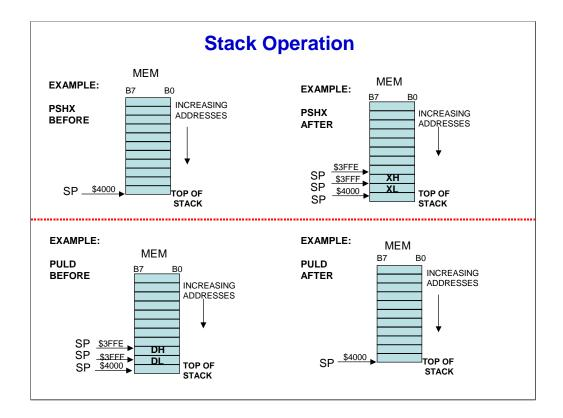
Here, you can see the Push operation depicted. Note that the SP is decremented by two and then the X register is pushed onto the stack.
