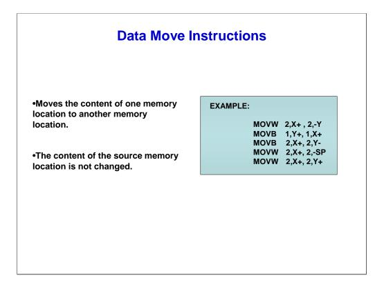
The function of the data move instructions is to move the content of one memory location to another memory location. As a result, the content of the source memory location is not changed.
