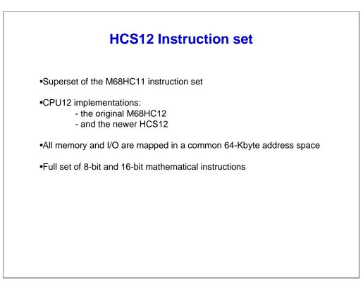
Let's start with the HCS12 instruction set. CPU12 instructions are a superset of the M68HC11 instruction set. Code written for an M68HC11 can be reassembled and runs on a CPU12 with no changes. The CPU12 provides expanded functionality and increased code efficiency.
