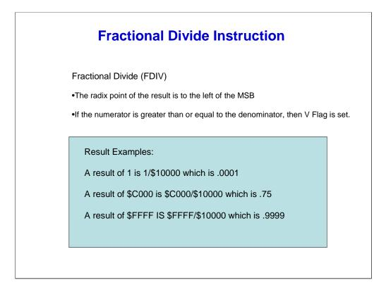
Here are the Fractional Divide (FDIV) instructions. FDIV may be executed after IDIV to resolve the remainder. In fact, FDIV can follow another FDIV to resolve more bits past the radix point. If the numerator is greater than or equal to the denominator, then V Flag is set which indicates an overflow condition is generated by this operation.
