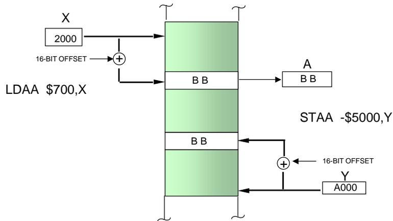
The third indexed addressing mode shown here uses 16-bit signed offset which is added to the index register (X, Y, SP or PC) allowing the CPU to access the memory location pointed to by the index register with an offset of up to +32K and -32K byte locations. This addressing mode, with 16-bit offset, allows the CPU to index to any memory location in the 64K memory map.
