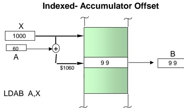
In this indexed addressing mode, the effective address is the sum of the values in the base index register and an unsigned offset in one of the accumulators. The value in the index register itself is not changed. The index register can be X, Y, SP, or PC. The accumulator can be either of the 8-bit accumulators (A or B) or the 16-bit D accumulator. The offset range can be up to + or – 32 Kbytes from base register.
