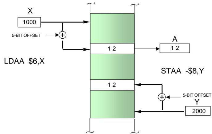
Now, let's look at some examples of the new indexed addressing modes available in the HCS12 instruction set. The first indexed addressing mode shown here uses an efficient short 5-bit signed offset allowing the CPU to access the memory location pointed to by the index register +15 and -16 byte location. The short 5-bit offset is added to the base index register (X, Y, SP, or PC) to form the effective address of memory location that will be affected by the instruction.
