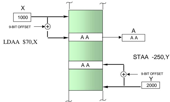
The second indexed addressing mode shown here uses 9-bit signed offset which is added to the index register (X, Y, SP or PC) allowing the CPU to access the memory location pointed to by the index register +255 and -256 byte location.
