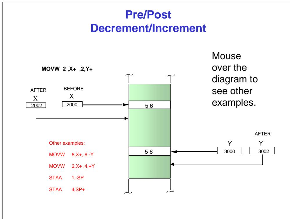
This indexed addressing mode provides four ways to automatically change the value in a base index register as a part of instruction execution. The index register can be incremented or decremented by an integer value either before or after indexing takes place. The base index register may be X, Y, or SP. Note that auto-modify modes would not make sense on PC.
