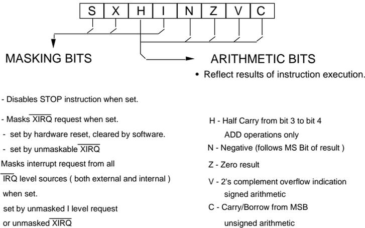
Now, let's look at the condition code register in more detail. Condition Code Flags reflect the results of arithmetic and other operations of the CPU as it performs instructions. These include H, Half Carry; N, Negative; Z, Zero; V, Overflow; and C, Carry/Borrow.
