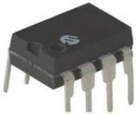
The MCP2551 is a high-speed CAN, fault-tolerant device that serves as the interface between a CAN protocol controller and the physical bus. The MCP2551 device provides differential transmit and receive capability for the CAN protocol. It will operate at speeds of up to 1 Mb/s. It also provides a buffer between the CAN controller and the high-voltage spikes that can be generated on the CAN bus by outside sources (EMI, ESD, electrical transients, etc.).
