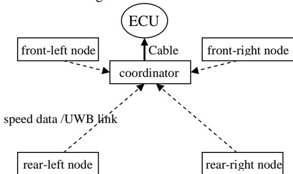
Figure 1. Star topology of the intra-vehicle UWB network
