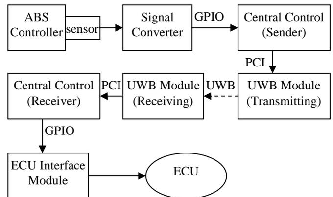
Figure 2. Testbed components and data flow
