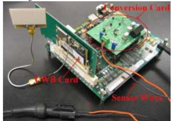
Figure 4. Central control, sensor signal conversion and UWB module assembly.
