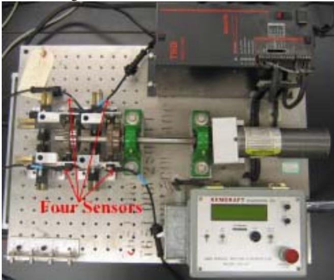
Figure 3. ABS motor control simulating system and wheel speed sensors
