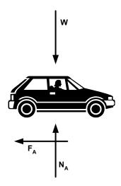
Because the road was assumed to be flat, the normal force, N<sub>A</sub>, is equal to the vehicle's weight.
